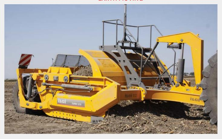
The Gated Ejector Construction series scraper is designed for soil transport and land leveling. It is equipped with a dual cylinder ejection system, one piece gate, and reinforced frame. The GECS series is designed to comply with higher horse powered tractors and heavier load capacities. The GECS series comes standard with a laser/GPS platform. It isequipped with tandem hydraulic hose kits to pull multiple scrapers behind a single tractor.
